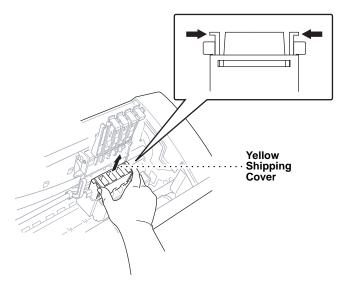
**4** Remove the yellow shipping cover by lifting it up and out.
